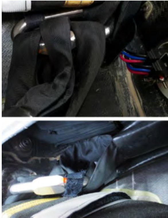
FIGURE 19-14 HARNESS ENDS INSERTED INTO 1/2" QUICK LINK
