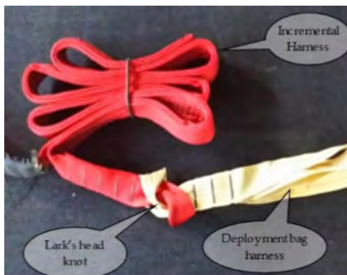
FIGURE 19-20 INCREMENTAL HARNESS TO DEPLOYMENT BAG STRAP
