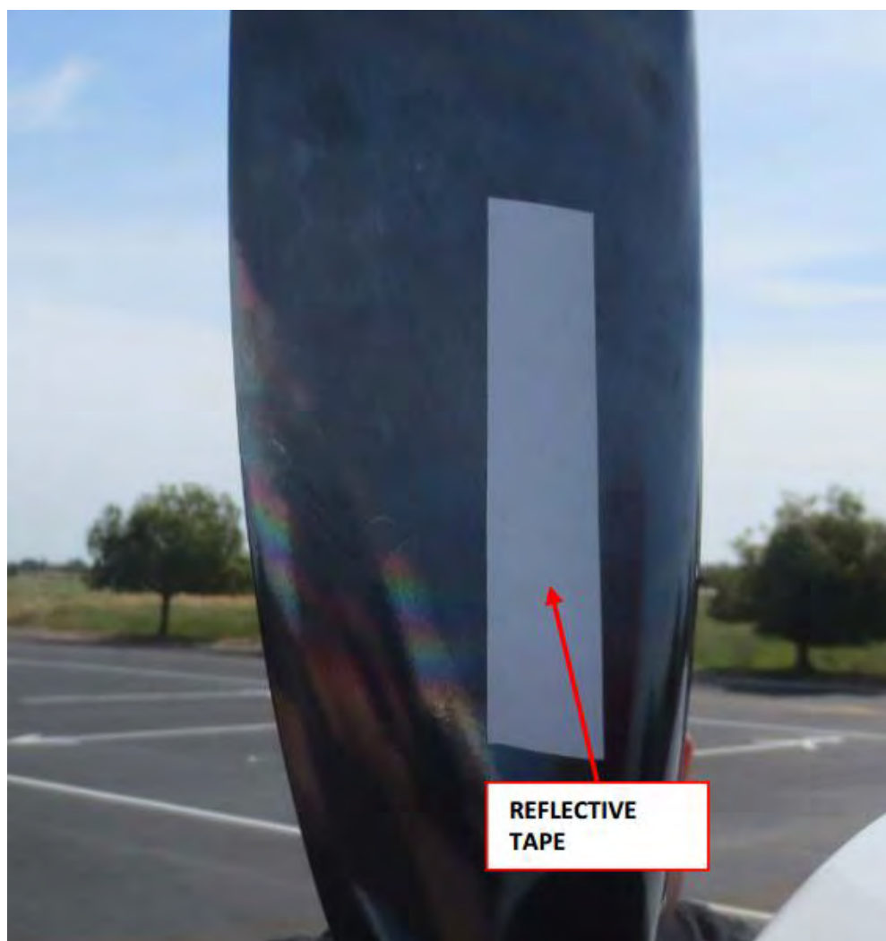
FIGURE 16-62 EXAMPLE OF REFLECTIVE TAPE PLACEMENT
