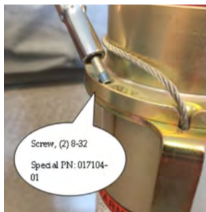
FIGURE 19-22 SECURING ROCKET COLLAR TO BRS 601 ROCKET TUBE
