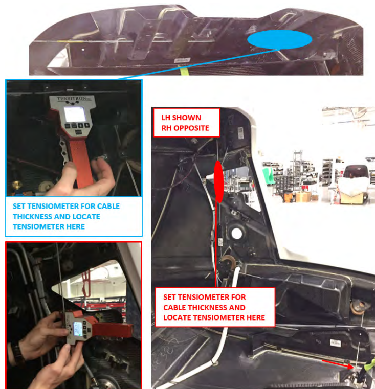
FIGURE 9-12 TENSIO METER LOCATIONS
