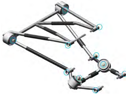
FIGURE 16-19 ENGINE MOUNT (RR, LH VIEW) WITH SCREW LOCATIONS CIRCLED IN BLUE
