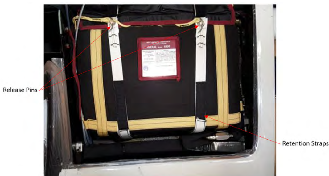
FIGURE 19-1 PARACHUTE PACKAGE INSIDE OF PARACHUTE BAY
