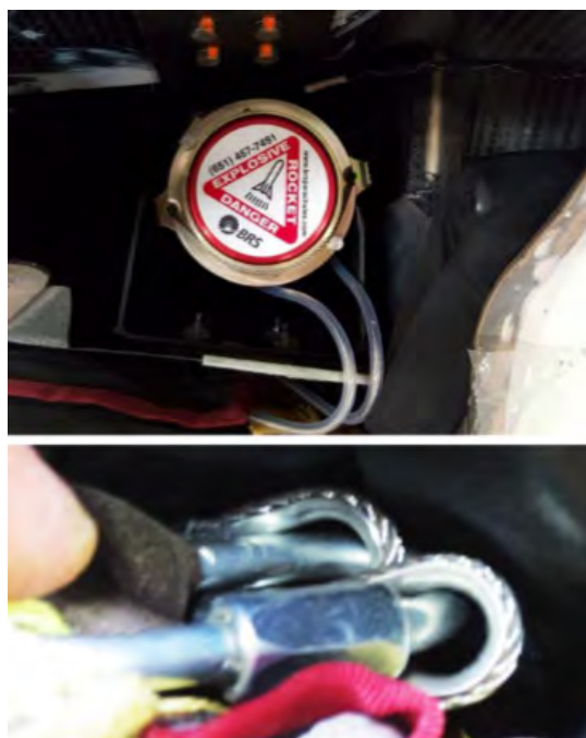
FIGURE 19-19 SECURING ROCKET COLLAR LANYARD AND INCREMENTAL HARNESS
