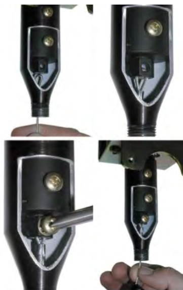
FIGURE 19-23 THREADING ACTIVATION CABLE LOOP
