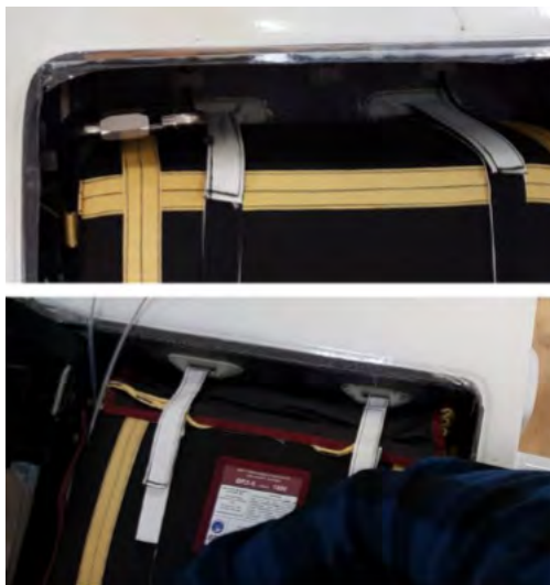
FIGURE 19-2 SECURING PARACHUTE DEPLOYMENT BAG
