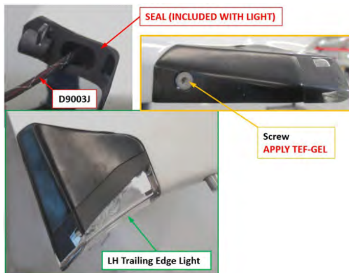
FIGURE 6-14 TRAILING EDGE LIGHT ASSEMBLY, LH
