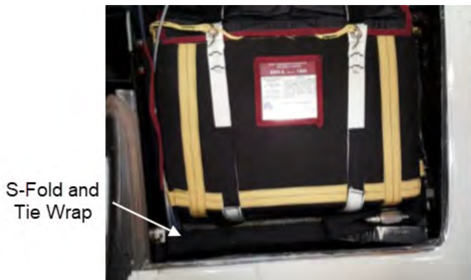
FIGURE 19-15 HARNESS INSTALLATION: "S"-FOLD AND TIE WRAP
