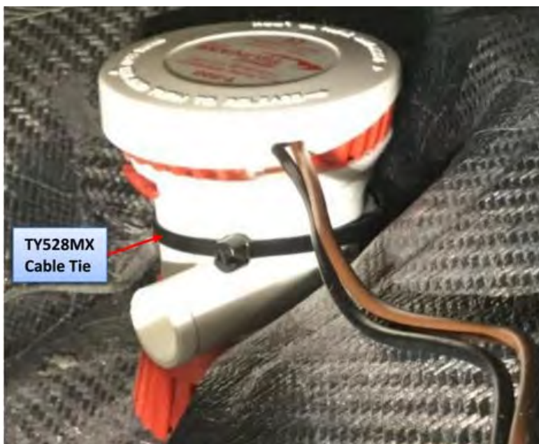
FIGURE 6-8 SECURE THE PUMP TO MOUNTING FLANGE
