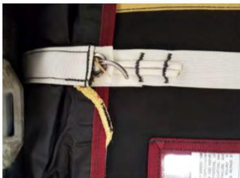
FIGURE 19-3 CURVED RELEASE PIN WITH TETHER
