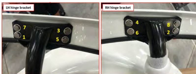
FIGURE 11-2 TORQUE ATTACHMENT BOLTS
