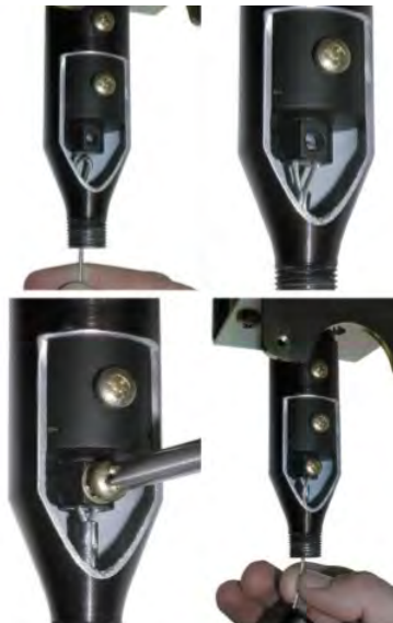
FIGURE 19-23 THREADING ACTIVATION CABLE LOOP
