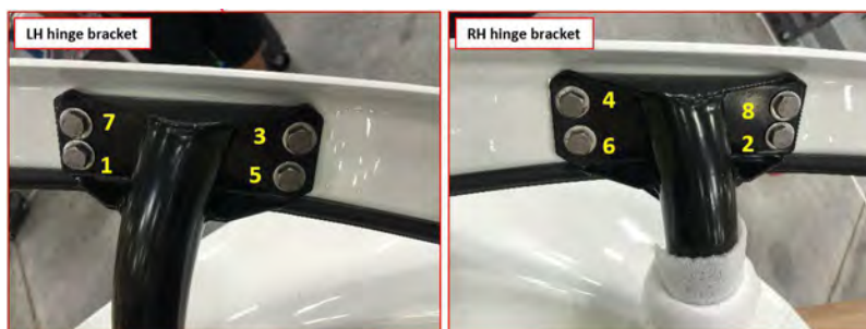
FIGURE 11-2 TORQUE ATTACHMENT BOLTS
