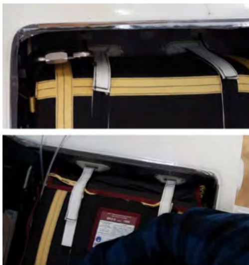
FIGURE 19-2 SECURING PARACHUTE DEPLOYMENT BAG
