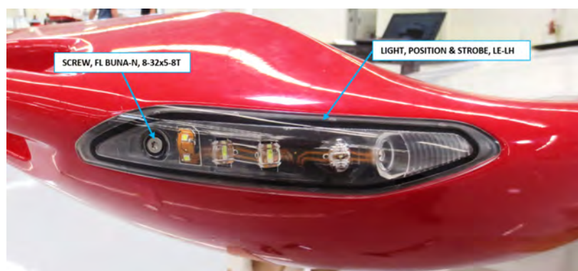
FIGURE 6-13 LEADING EDGE LIGHT ASSEMBLY, LH
