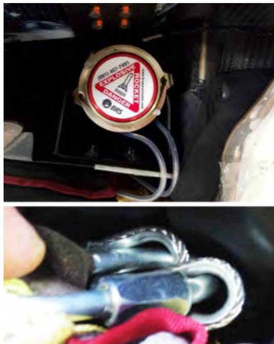
FIGURE 19-19 SECURING ROCKET COLLAR LANYARD AND INCREMENTAL HARNESS
