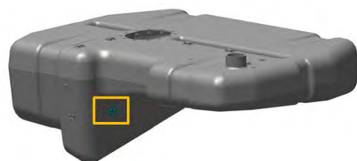
FIGURE 10-12 CABLE TIE ANCHOR MOUNT EXTERIOR LOCATIONS 6&7
