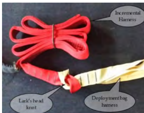
FIGURE 19-20 INCREMENTAL HARNESS TO DEPLOYMENT BAG STRAP
