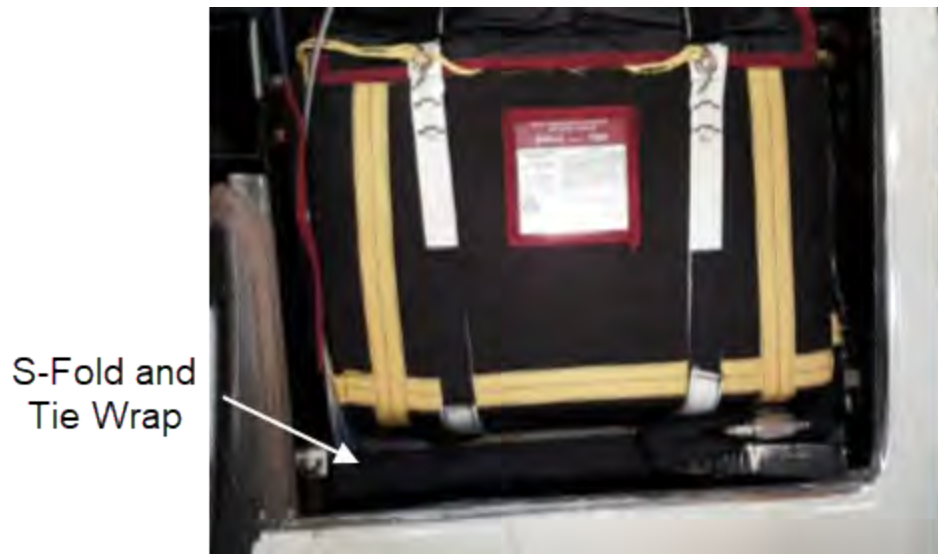
FIGURE 19-15 HARNESS INSTALLATION: "S"-FOLD AND TIE WRAP
