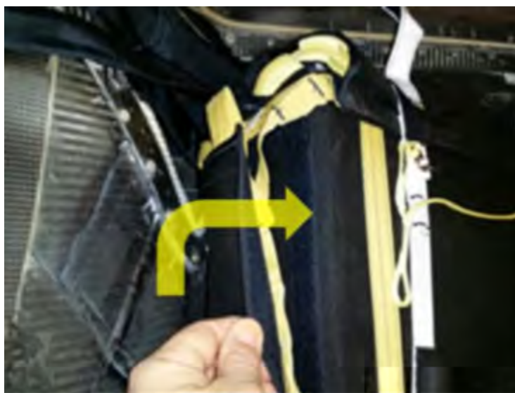
FIGURE 19-5 SIDE FLAP CONTAINING COLLAR LINE AND INCREMENTAL HARNESS
