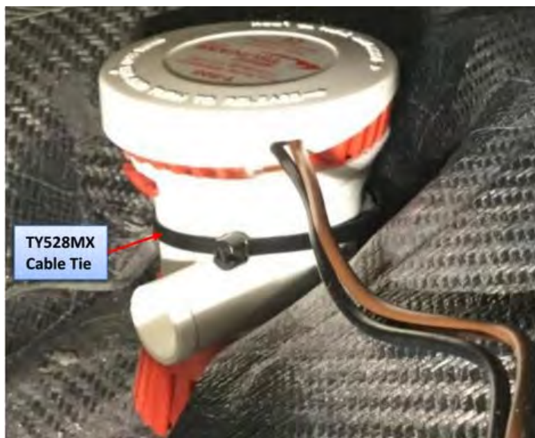
FIGURE 6-8 SECURE THE PUMP TO MOUNTING FLANGE
