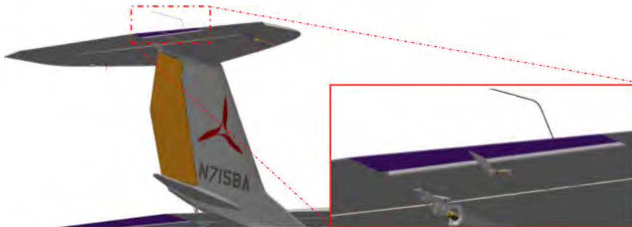
FIGURE 9-40 PITCH TRIM TAB AND VERTICAL TAIL
