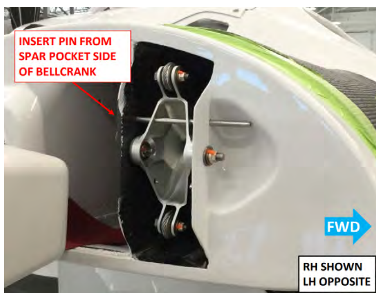
FIGURE 9-11 WING SOCKET BELLCRANK RIG PIN LOCATION
