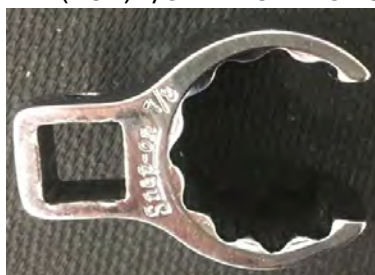
FIGURE 16-10 METHOD A VS. METHOD B (TOP) 7/8" 12-POINT CROWS FOOT WRENCH (BOTTOM)
