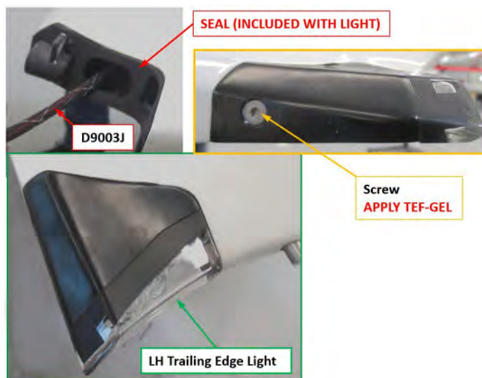
FIGURE 6-14 TRAILING EDGE LIGHT ASSEMBLY, LH
