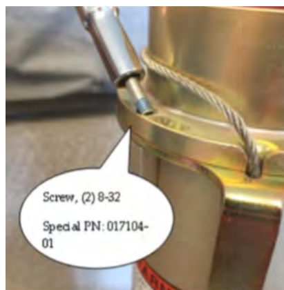
FIGURE 19-22 SECURING ROCKET COLLAR TO BRS 601 ROCKET TUBE
