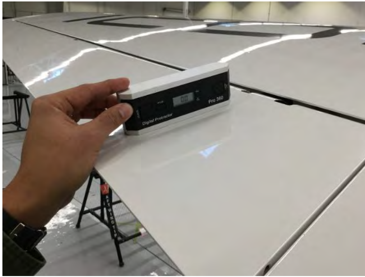
FIGURE 9-19 AILERON DIGITAL PROTRACTOR
