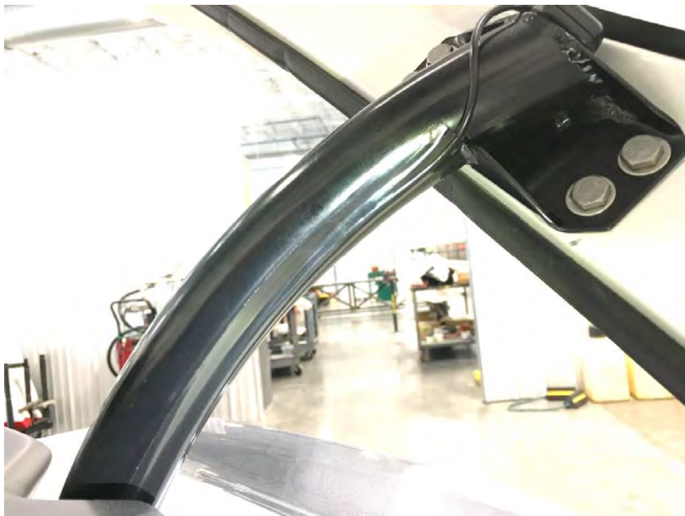
FIGURE 13-26 ANTENNA ROUTING LOOKING LEFT, OUTBOARD. CANOPY OPEN
