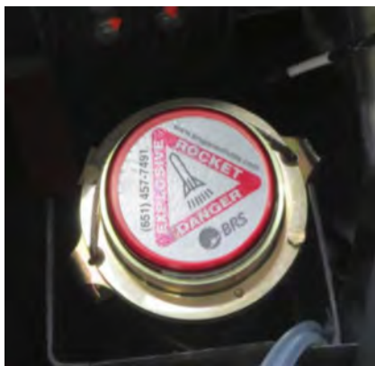
FIGURE 19-16 SECURE ROCKET TO ICON A5 ROCKET MOUNT BRACKET
