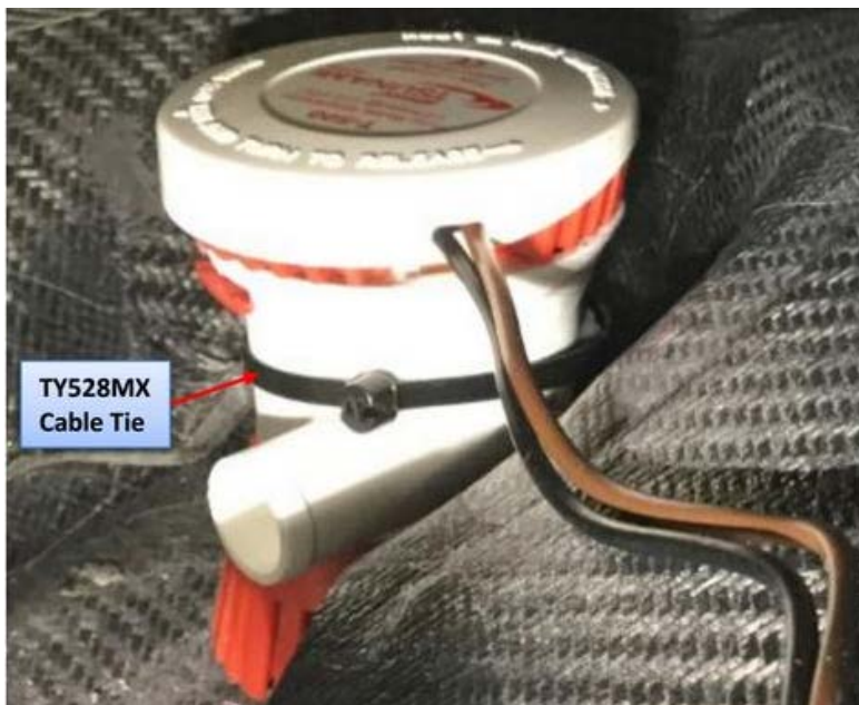
FIGURE 6-11 SECURE THE PUMP TO MOUNTING FLANGE
