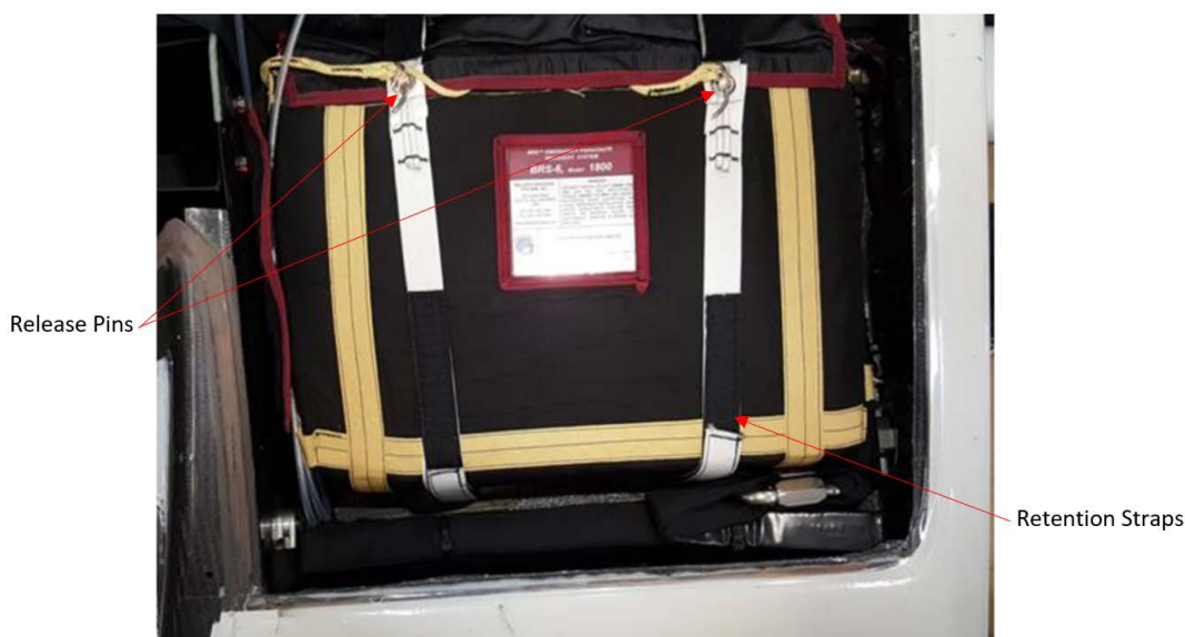
FIGURE 19-1 PARACHUTE PACKAGE INSIDE OF PARACHUTE BAY
