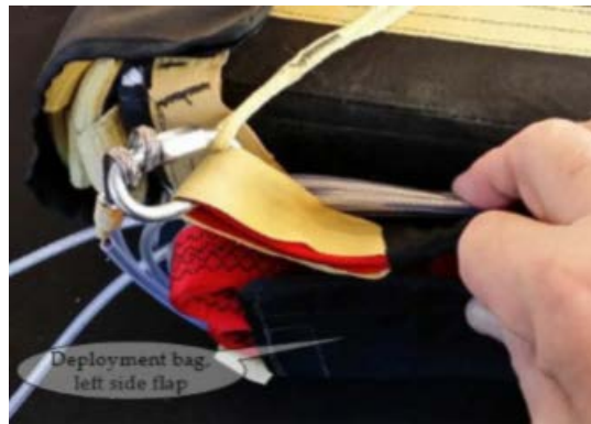
FIGURE 19-21 DEPLOYMENT BAG, LEFT SIDE FLAP
