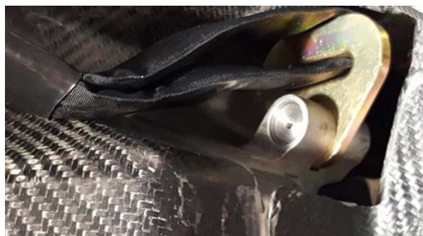
FIGURE 19-8 “A” END OF HARNESS ATTACHMENT POINT (STARBOARD FORWARD)
