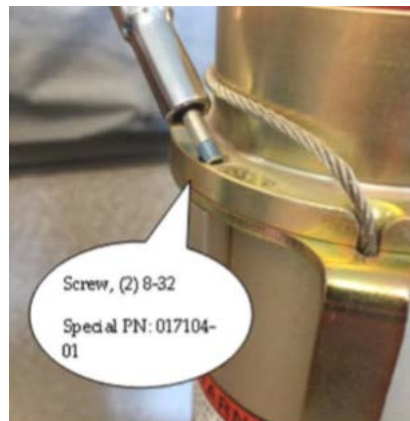
FIGURE 19-22 SECURING ROCKET COLLAR TO BRS 601 ROCKET TUBE
