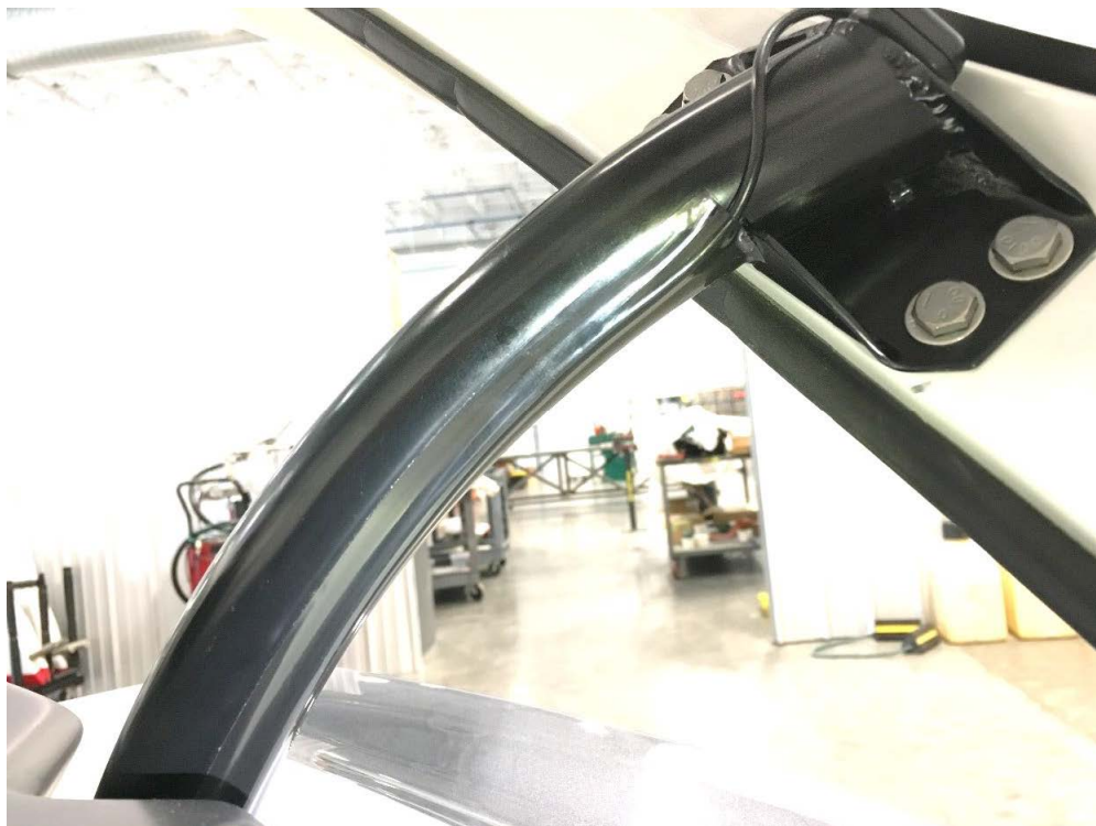
FIGURE 13-57 ANTENNA ROUTING LOOKING LEFT, OUTBOARD. CANOPY OPEN
