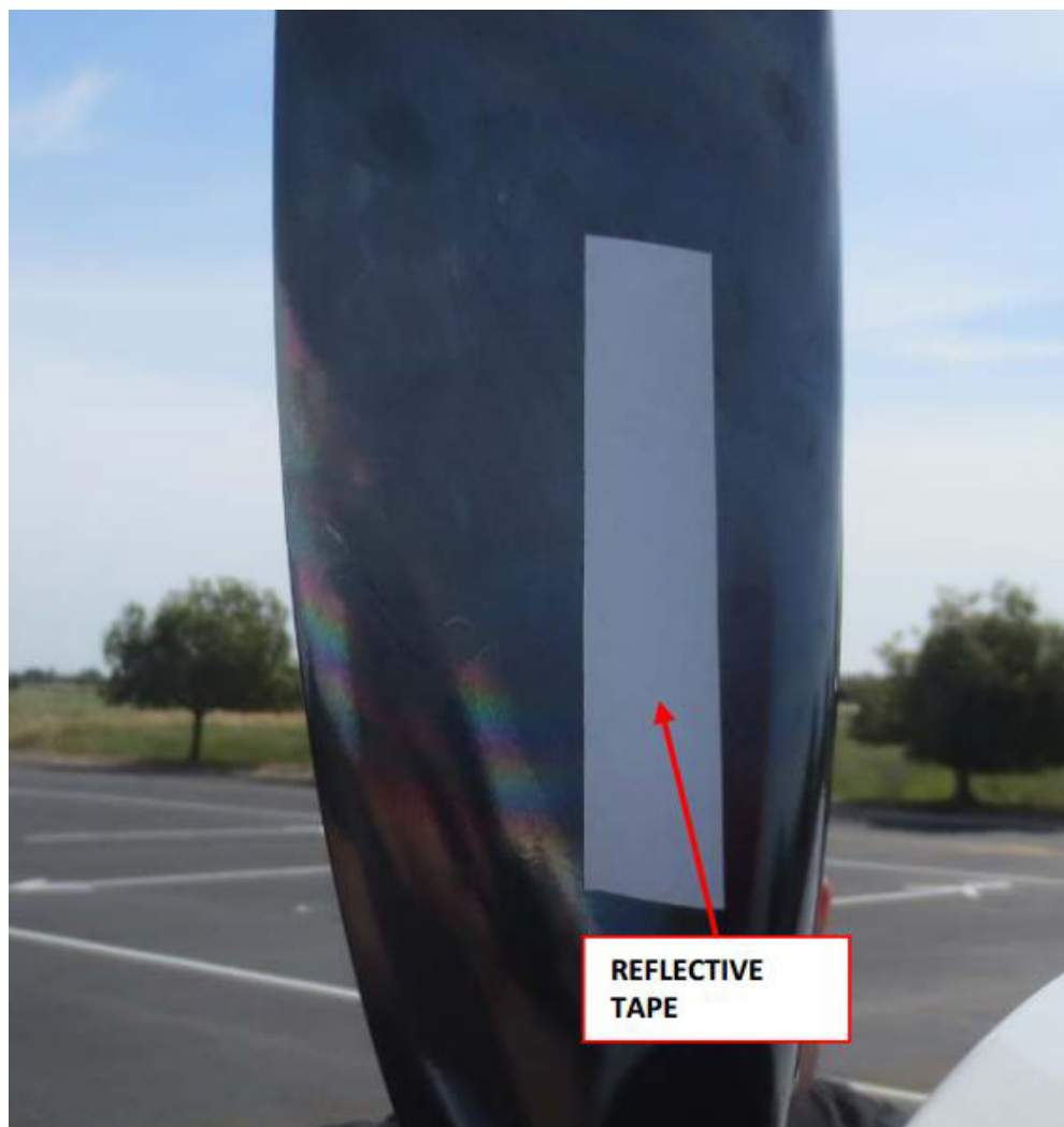
FIGURE 16-67 EXAMPLE OF REFLECTIVE TAPE PLACEMENT
