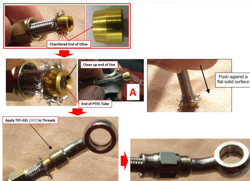
FIGURE 14-17 GENERAL BRAKE LINE TERMINATION
