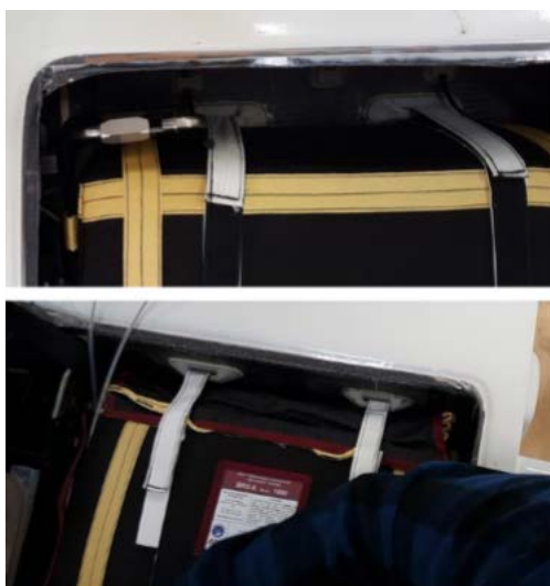
FIGURE 19-2 SECURING PARACHUTE DEPLOYMENT BAG
