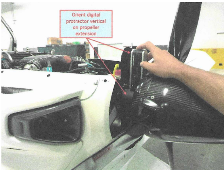
FIGURE 16-72 CALIBRATE DIGITAL PROTRACTOR
