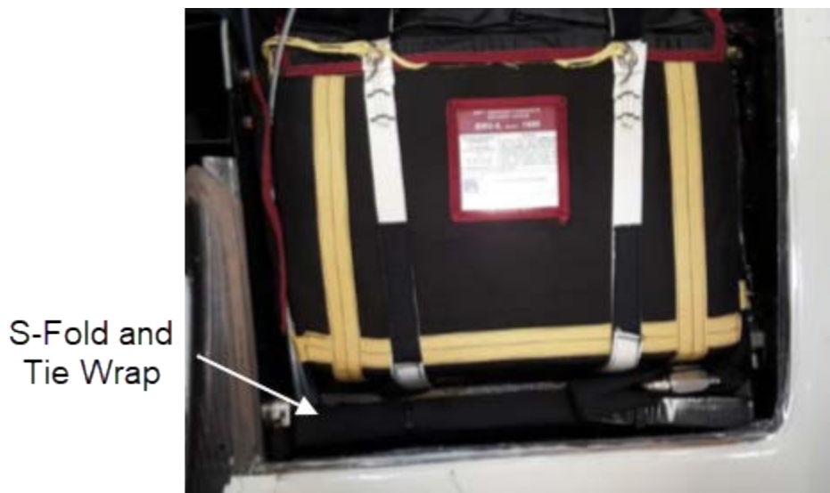
FIGURE 19-15 HARNESS INSTALLATION: "S"-FOLD AND TIE WRAP
