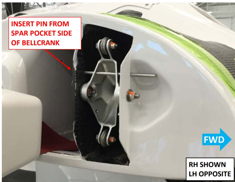
FIGURE 9-11 WING SOCKET BELLCRANK RIG PIN LOCATION
