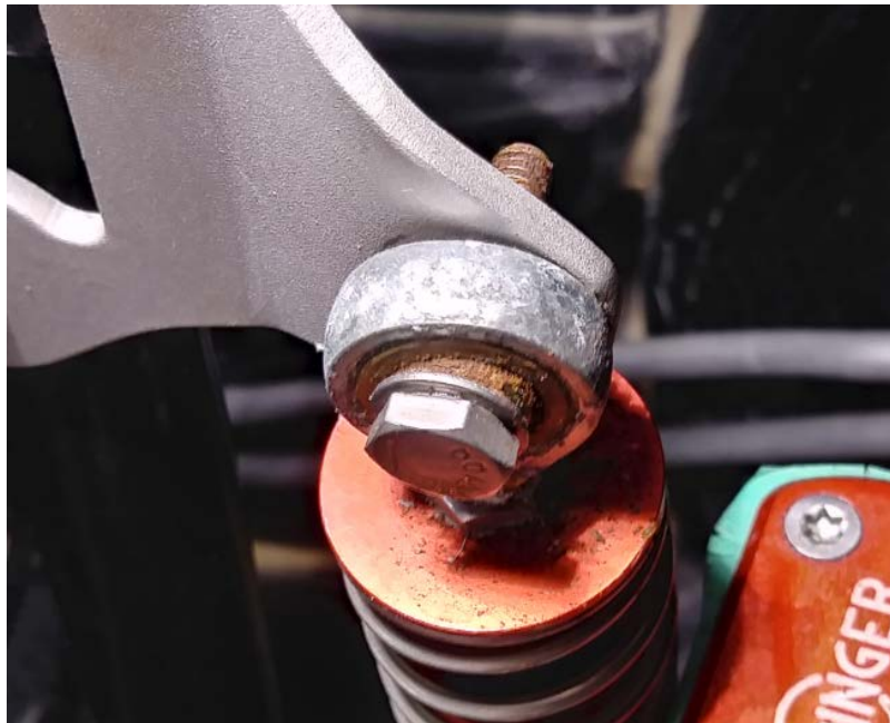
Figure 2: Unacceptable Corrosion on rod end.
