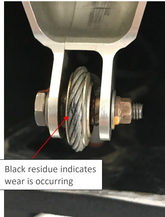
Figure 4: Black residue indicating wear
