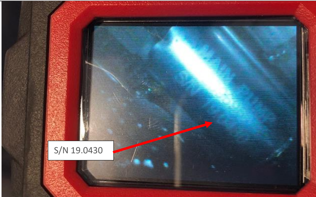
Figure 5: View of the borescope screen showing the fuel pump serial number.
