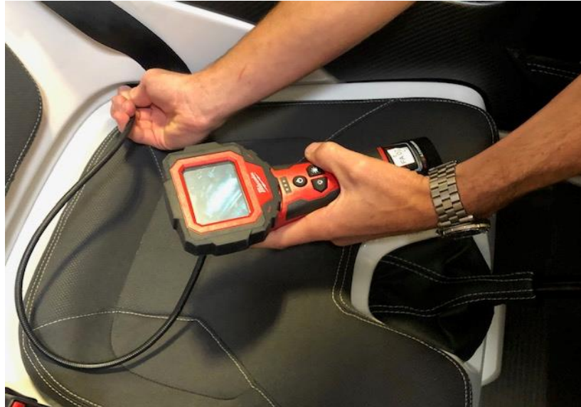
Figure 3: Borescope inspection technique through the pilot side lap belt pass through
