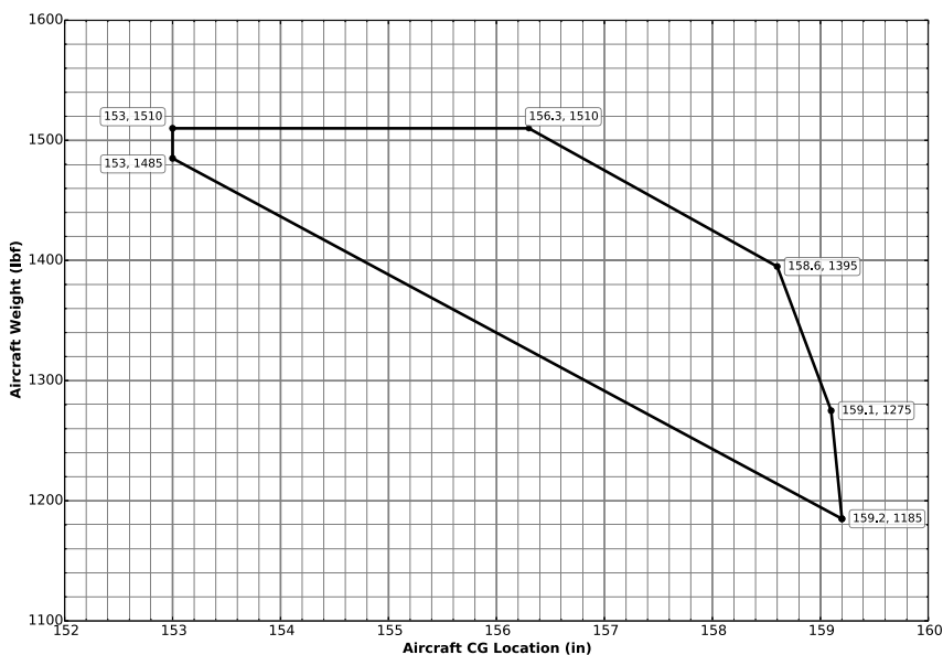
FIGURE 6-2 WEIGHT AND CG ENVELOPE LIMITS
