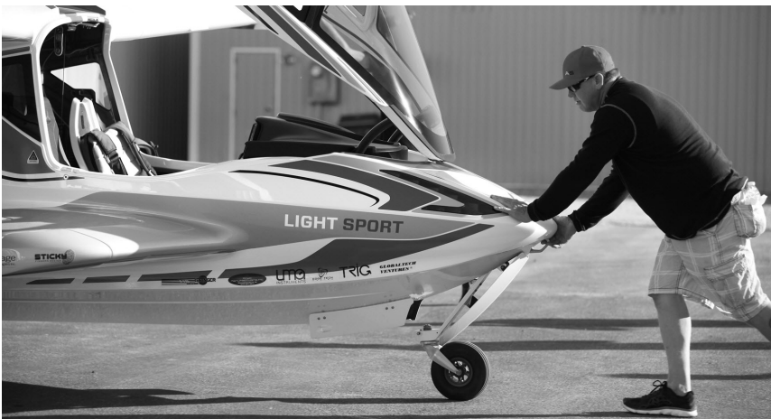
FIGURE 8-1 APPROPRIATE GROUND HANDLING TECHNIQUE
