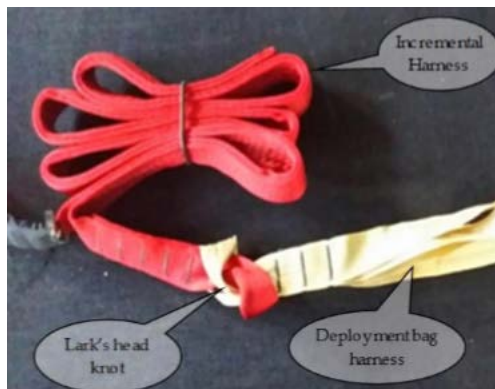
FIGURE 19-20 INCREMENTAL HARNESS TO DEPLOYMENT BAG STRAP
