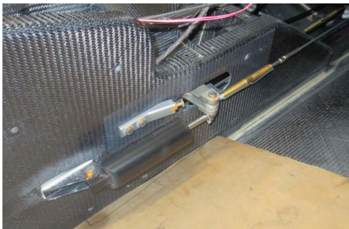
FIGURE 9-55 RUDDER RETURN SPRING
