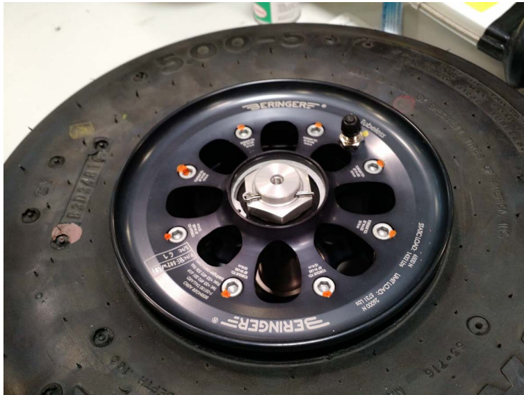
FIGURE 14-25 WHEEL NUT DETAIL.
