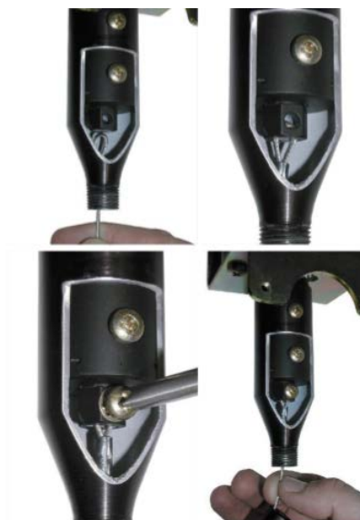
FIGURE 19-23 THREADING ACTIVATION CABLE LOOP
