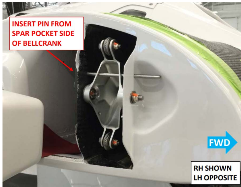
FIGURE 9-11 WING SOCKET BELLCRANK RIG PIN LOCATION
