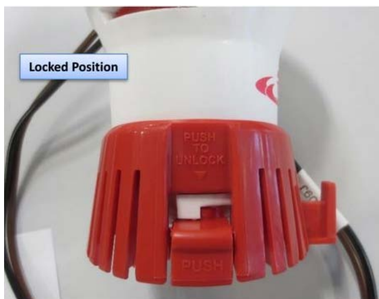
FIGURE 6-10 LOCK BOTTOM STRAINER
