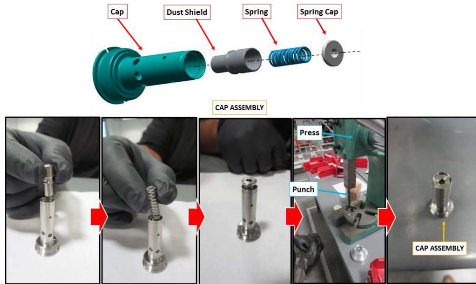
FIGURE 18-7 CAP ASSEMBLY
