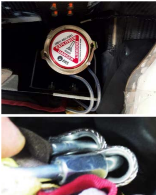
FIGURE 19-19 SECURING ROCKET COLLAR LANYARD AND INCREMENTAL HARNESS
