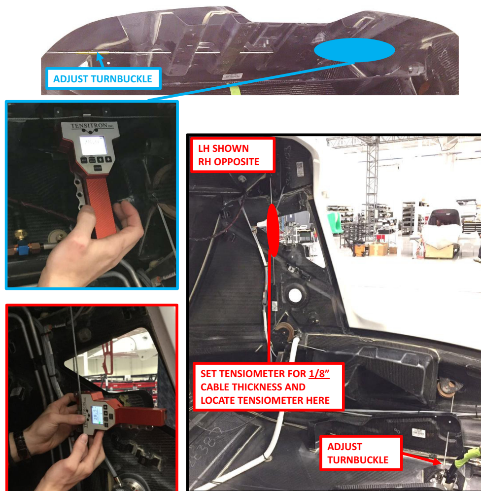
FIGURE 9-17 TENSIOMETER AND CABLE ADJUSTMENT LOCATIONS
