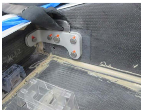
FIGURE 19-7 “A” END OF HARNESS ATTACHMENT POINT (STARBOARD REAR)
