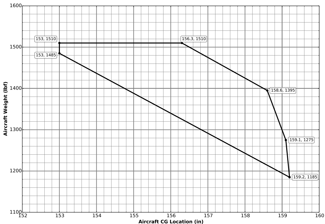
FIGURE 3-2 WEIGHT AND CG ENVELOPE LIMITS
