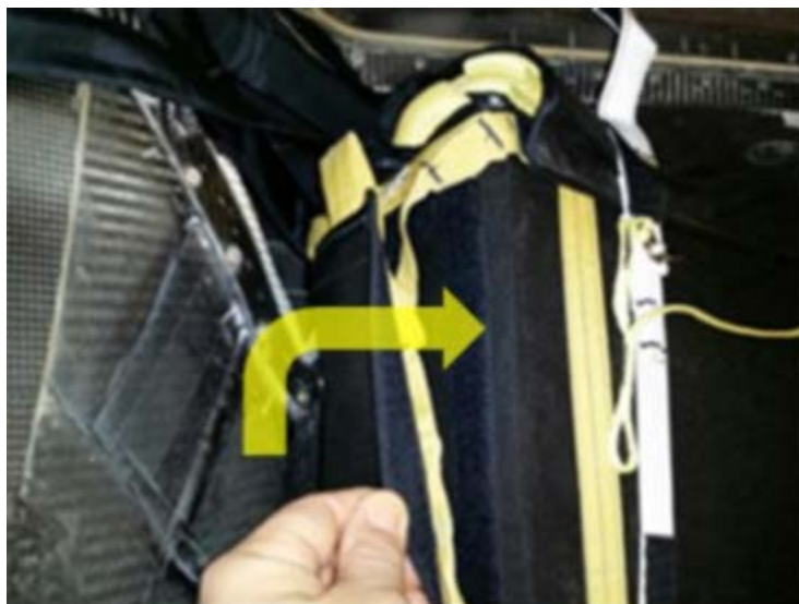
FIGURE 19-5 SIDE FLAP CONTAINING COLLAR LINE AND INCREMENTAL HARNESS
