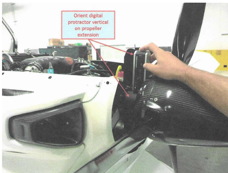
FIGURE 16-72 CALIBRATE DIGITAL PROTRACTOR
