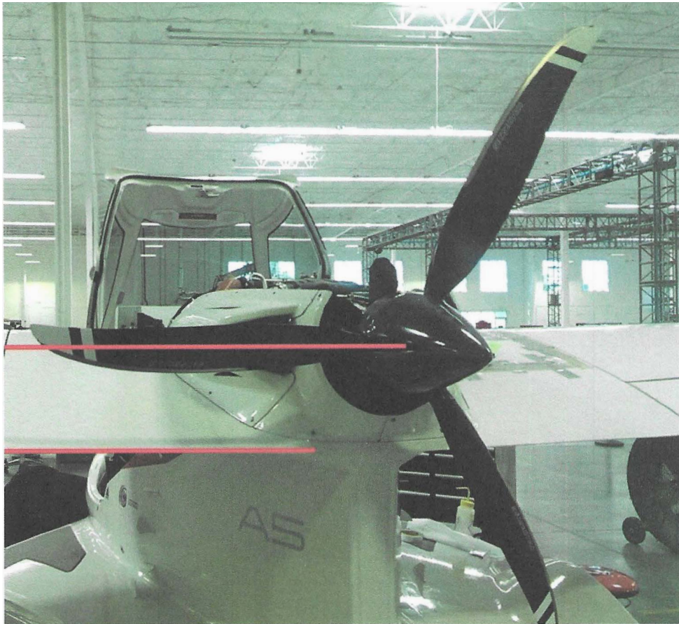
FIGURE 16-71 BLADE ORIENTATION TO THE GROUND
