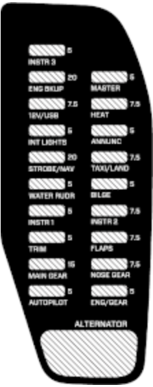
FIGURE 13-10 FUSE PANEL, AUTOPILOT CONFIGURATION
