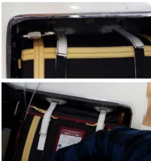
FIGURE 19-2 SECURING PARACHUTE DEPLOYMENT BAG
