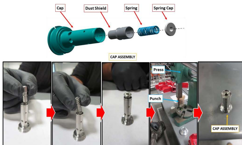
FIGURE 18-10 CAP ASSEMBLY
