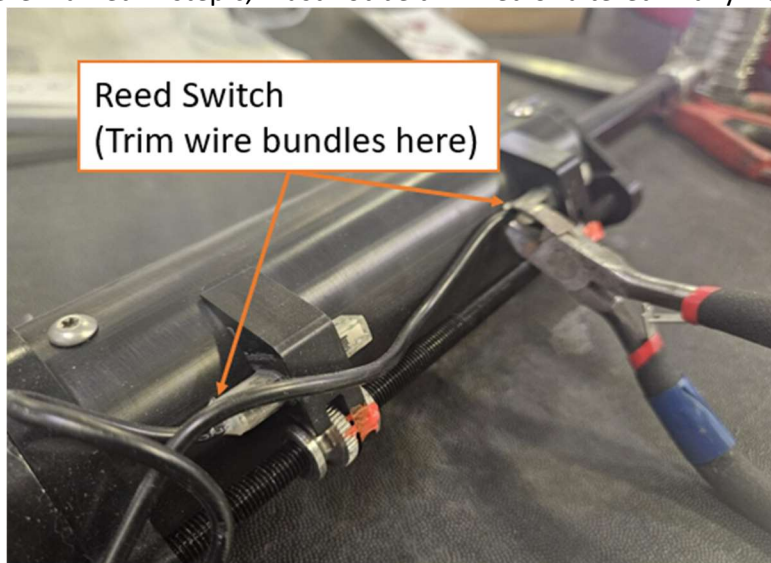
Figure 2. Trim wires at reed switches
