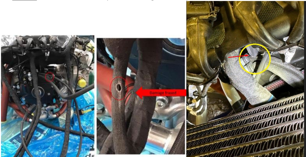
Figure 1. Location of Damaged Sleeving
