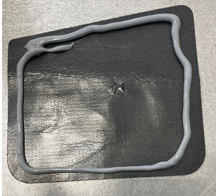
Figure 7 Wing fold tube cover with 3M Fire Barrier applied.
