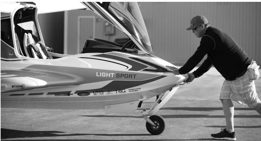
FIGURE 8-1 APPROPRIATE GROUND HANDLING TECHNIQUE
