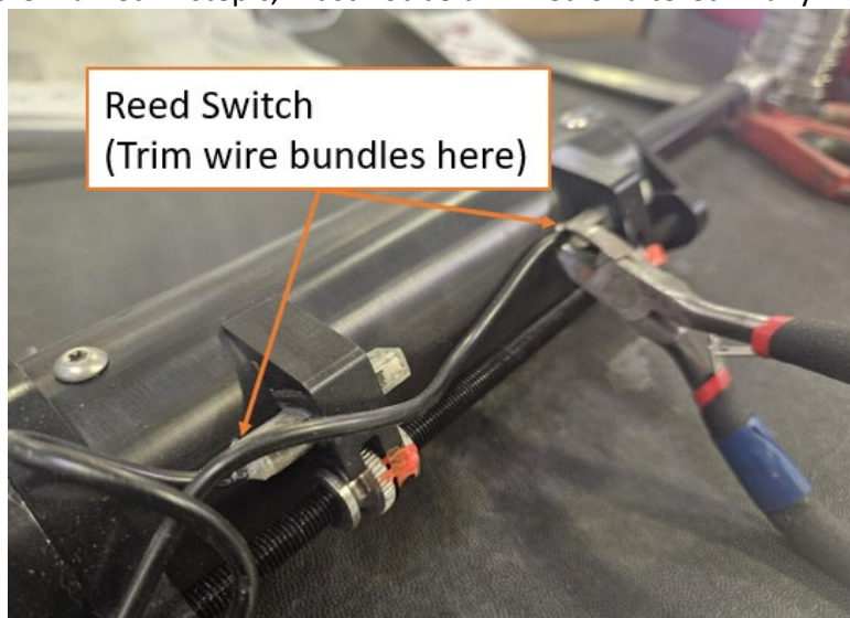
Figure 6. Trim wires at reed switches
