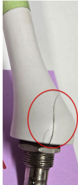
Figure 1. Examples of Cracks in Antenna Base
