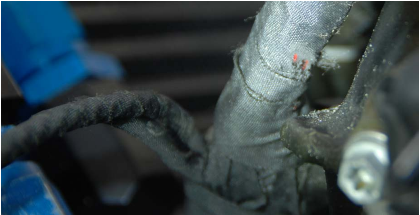
Figure 1. Engine wire harness damage due to chaffing
