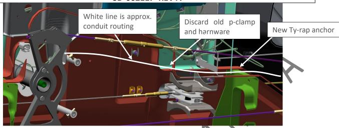
3. Terminate the throttle lever side of the conduit using the following method. Use a metal cut off wheel or a metal cutting hand saw to cut the conduit. DO NOT use side cutters. Use MA830 plexus adhesive for the epoxy and Loctite 243 on threads of the set screws.
